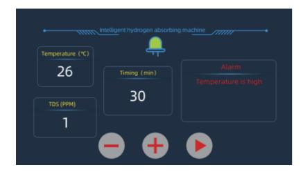
Alarm reason: The temperature inside the chassis reaches up to 60 °C and the display temperature is high.
