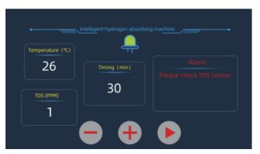
Alarm reason: adding impure water, or the water containing salt
