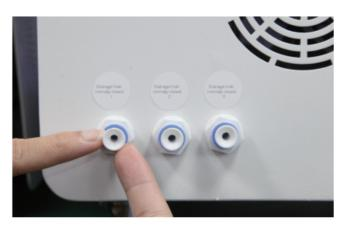
Drainage method: Press the blue ring backward with the index finger of your left hand, and at the same time, pull out the white plug with the index finger of your right hand forward, that is, drain the water. After drainage is completed, insert the white plug back into the drainage hole to close it.
