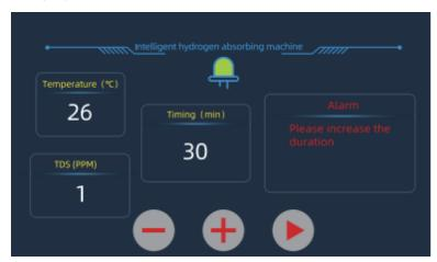
Alarm reason: TDS sensor is not recognized. There may be an internal blockage (please drain water from drain outlet 1-2 times, then add water to start the machine again) or the TDS sensor is damaged.
