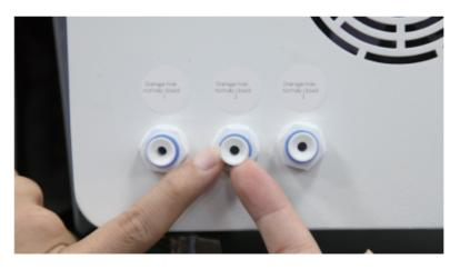
Solution: Close drain holes one and three, remove the plug of drain hole two to drain, then refill the water tank, and repeat the above operation 2-3 times.
